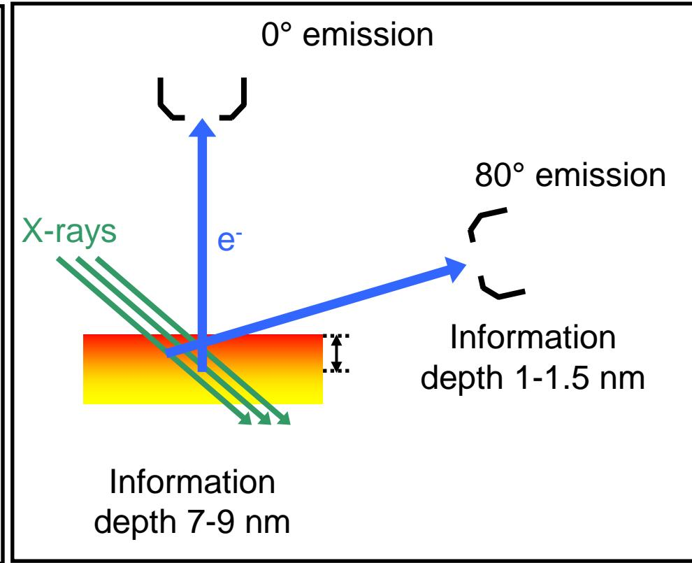
How to measure ARXPS without tilting a liquid sample?
