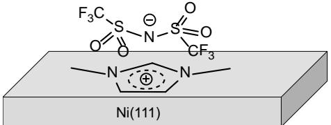
0.7 ML  $[C_1C_1Im][Tf_2N]$  on  $Ni(111)$
