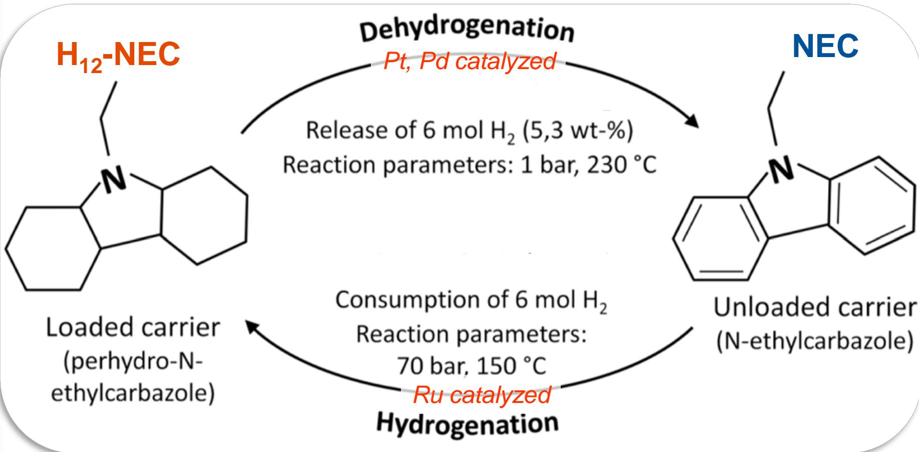
Reversible hydrogenation (Ru) and dehydrogenation (Pt, Pd) of N-ethylcarbazole (NEC) and perhydro-N-ethylcarbazole ( $H_{12}$ -NEC)
