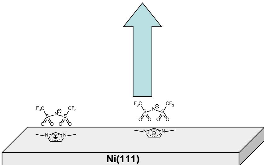
→ Rearrangement to **checkerboard** structure at higher film thickness
