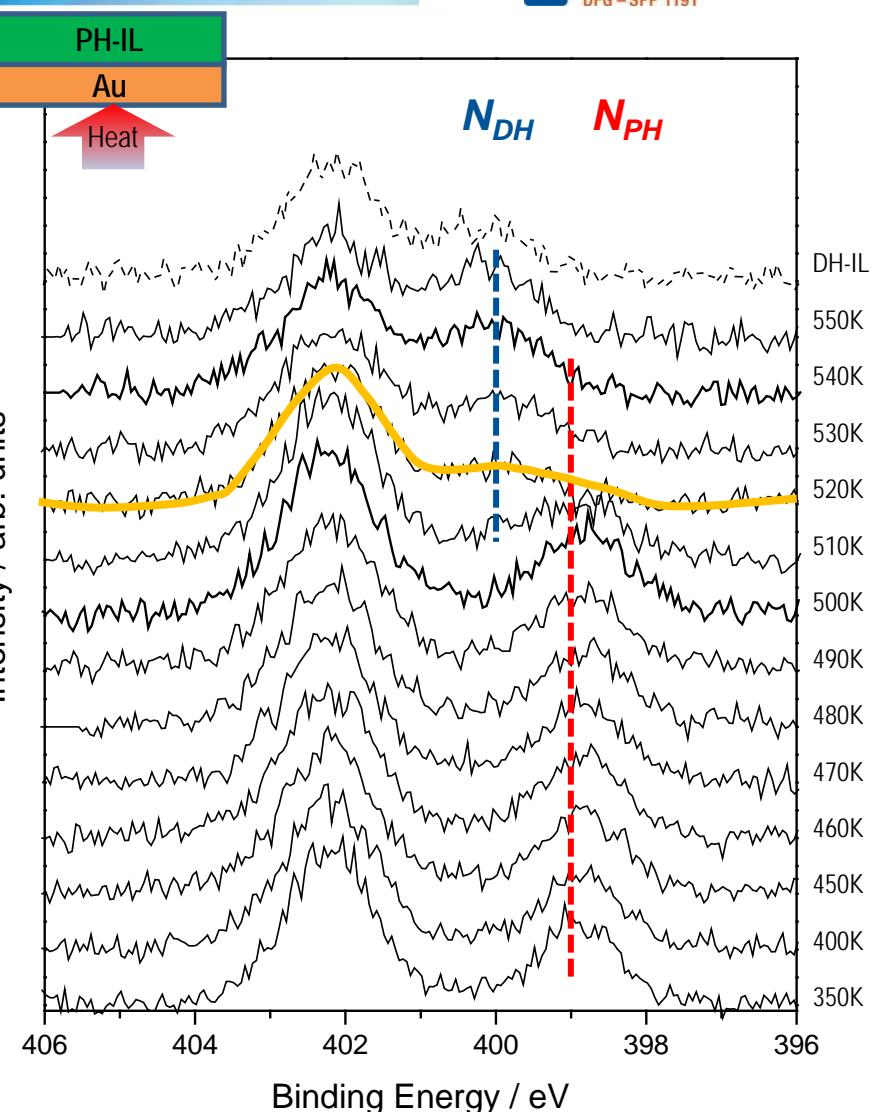
→ no catalyst (Au support): dehydrogenation & decomposition at  $T \geq 510\text{K}$
