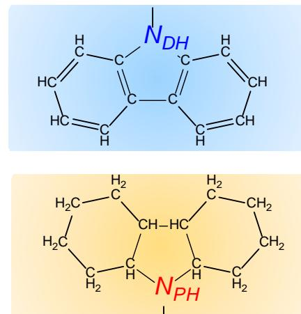
→ dehydrogenation liquid  $H_{12}$ -NEC (supported Pt @ 500K)
